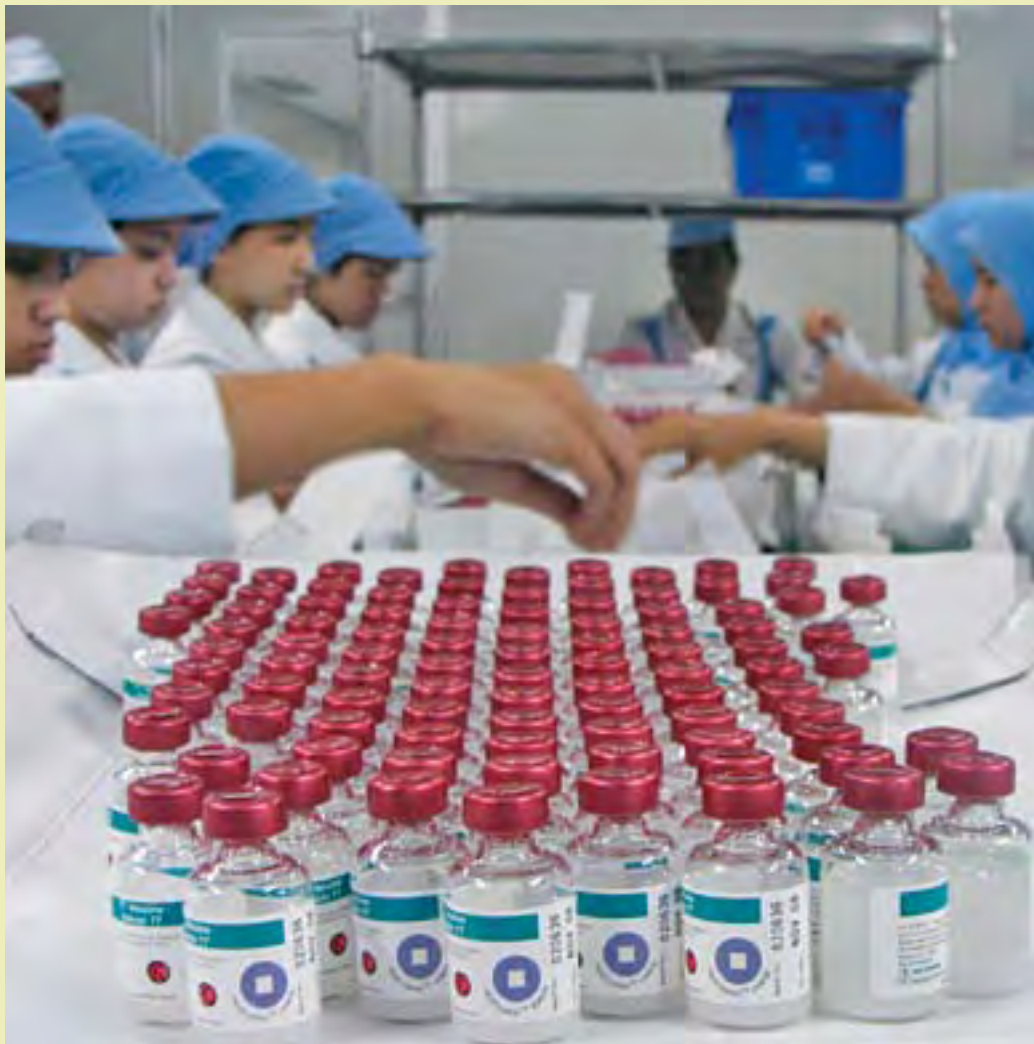
Vaccine vial monitors are dime-sized stickers that adhere to vaccine vials and change color as the vaccine is exposed to heat, letting health workers know whether the vaccine is still viable (4 billion units sold). Photo: World Health Organization/Umit Kartoglu
