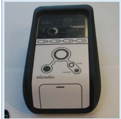
Prototype of the DxBox instrument with a disposable device.
